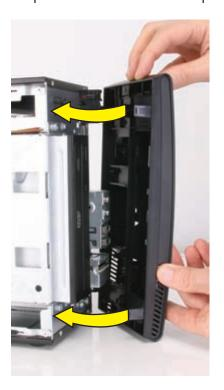
**13** Align the tabs on the inside edge of the left side panel with the slots in the edge of the left side of the computer case.
